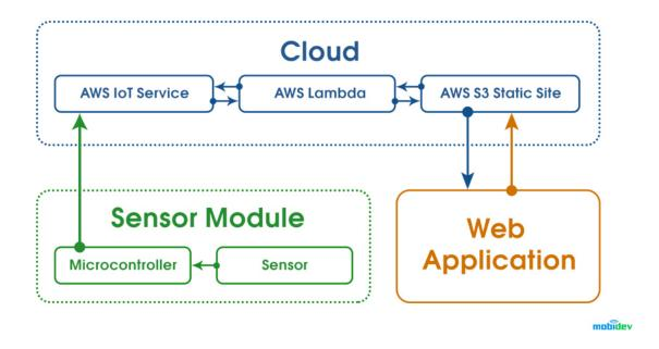
The IoT device consists of an ESP8266 microcontroller and an HC-SR04 distance measurement sensor. The sensor periodically measures the distance and transmits this data to the microcontroller, which is connected to AWS IoT service via the MQTT protocol.
